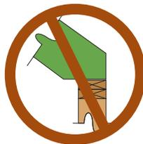
**Do not** overhang seat cuts on West Fraser™ LVL beams from inside face of support member
