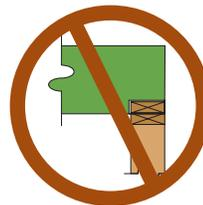
**Do not** notch underside of beam at bearing location
